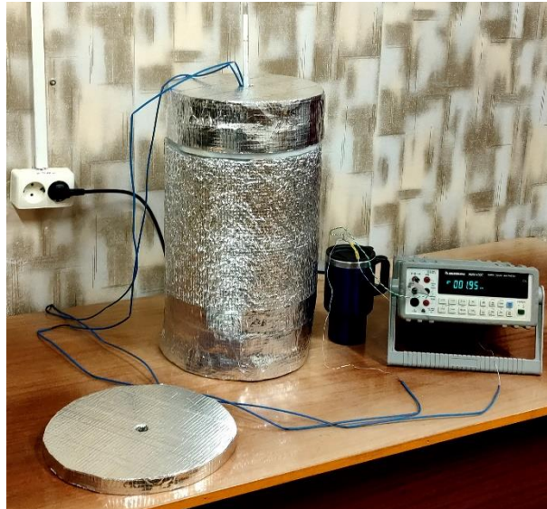
Fig. 2. Experimental unit for thermocouple calibration with expedient insulation radius
